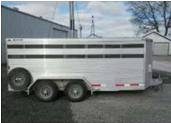
Standard stock trailer for transporting pigs, equipped with non-slip rubber floor and gates for separating individual pigs, or groups of pigs, during transport.
